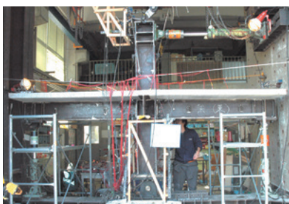
Experiment on semi-rigid composite connection (Study on composite structures by Assoc. Prof. Ohtani)
