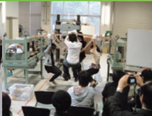
Practical design and fabrication of Wood Trusses. Students verified the strength using their own weight.
