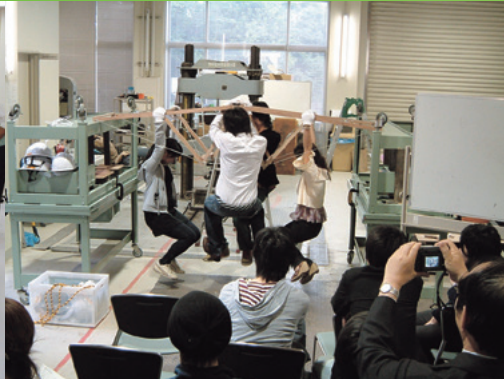
Practical design and fabrication of Wood Trusses. Students verified the strength using their own weight.
